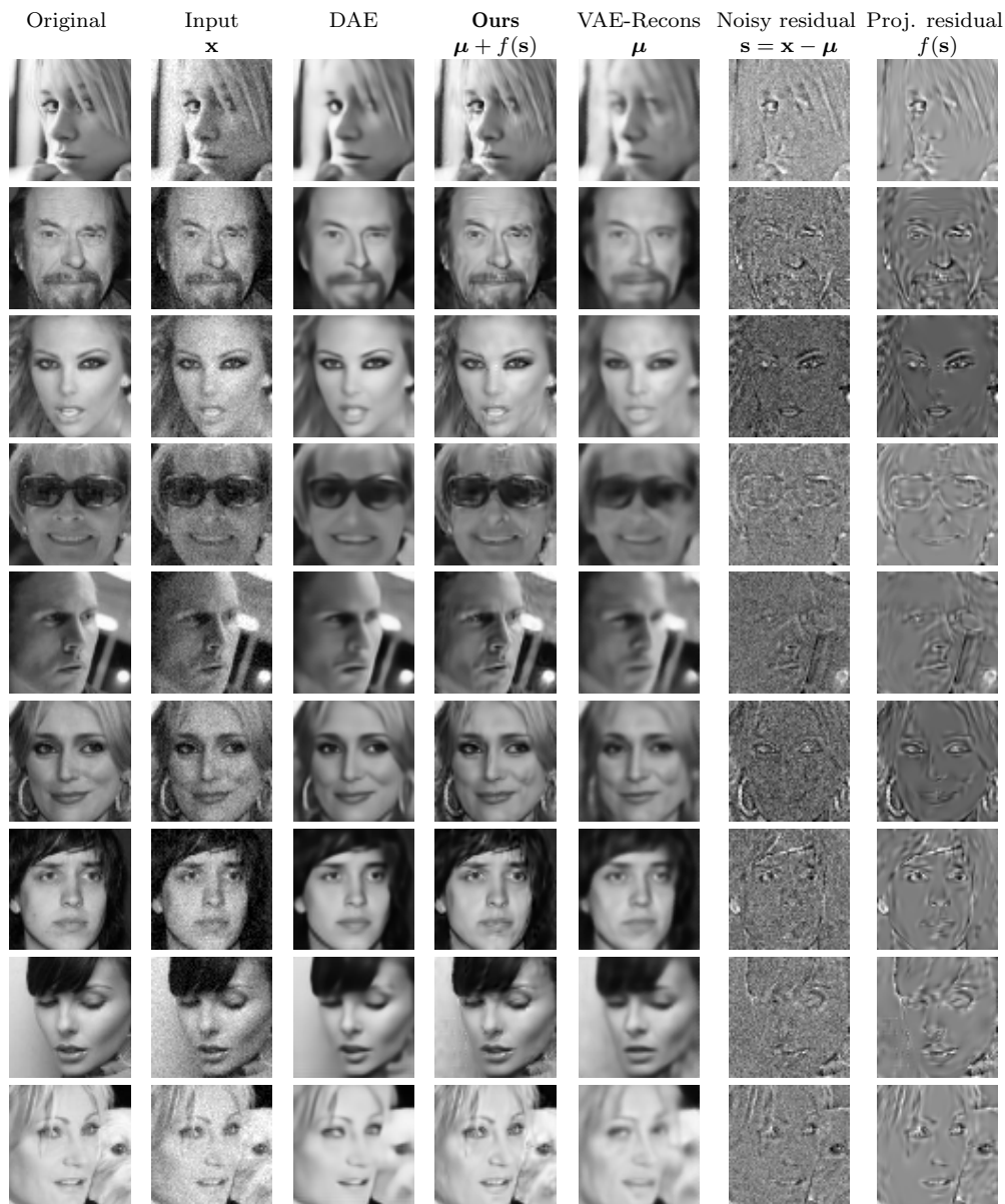
Figure A-20: Denoising experiment, left column: original image without noise, second column: image with added noise, third column: denoising autoencoder (DAE) result, fourth column: our result, fifth column: VAE reconstruction from the noisy input, sixth column: residual between the VAE reconstruction and the noisy input, right column: the noisy residual projected on \hat{\Sigma} , the matrix constructed with 1000 eigenvectors of \Sigma . Our result is the sum of the projected residual and the VAE reconstruction. Our model is able to recover fine details that are lost with the DAE approach.
