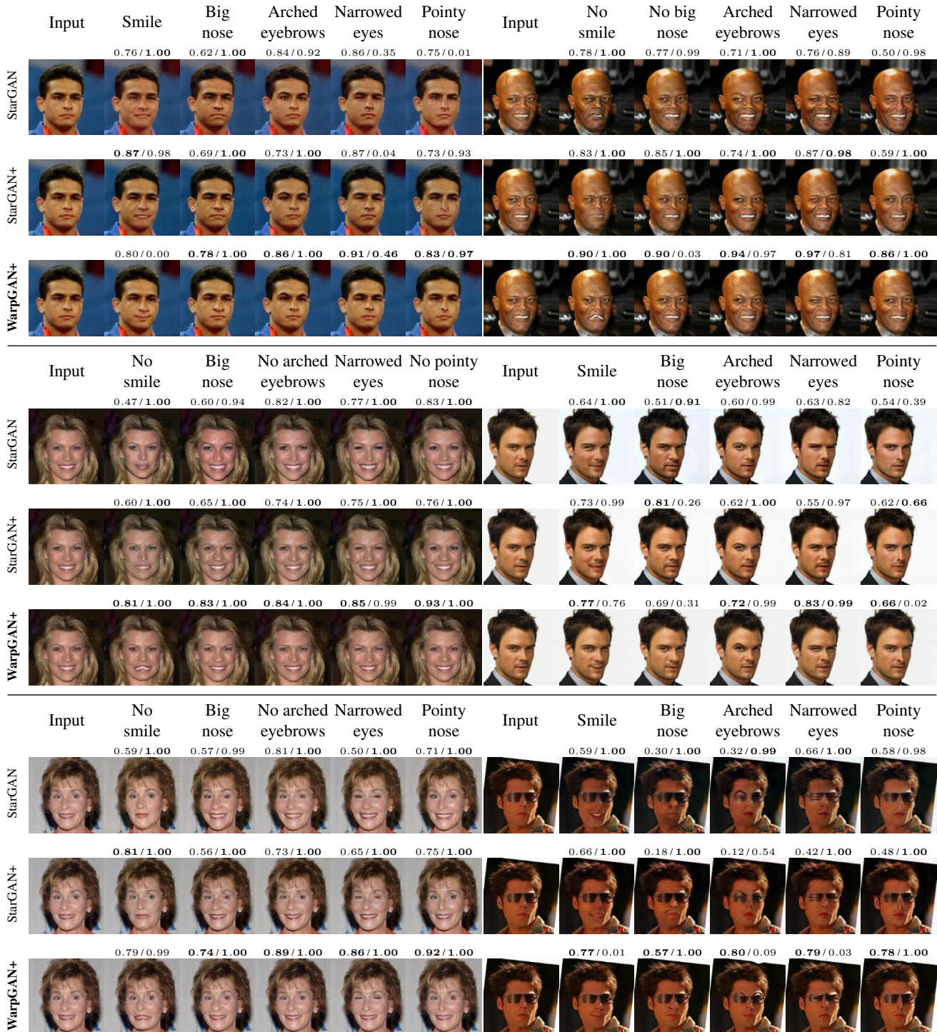
Figure 3: Comparison to previous work on the CelebA dataset. From a given input image, first column, each method attempts to transfer the semantic attribute in its corresponding column. On top of each image the re-identification score and the classification accuracy are shown as (id / cls) (higher is better). (Zoom in for details)
