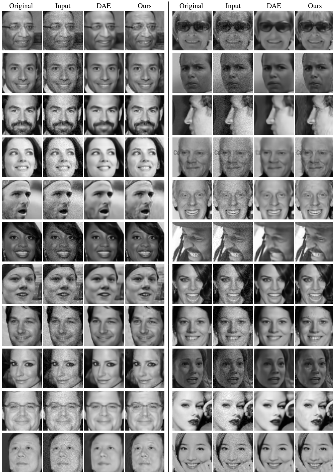
Figure 8: Denoising experiment, left column: original image without noise, second column: image with added noise, third column: denoising autoencoder result, and right column: our result. Our model is able to recover fine details with its structure residual prediction.
